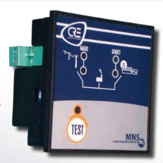
The MNS is a basic, microprocessor controlled unit designed to monitor 3-phase mains voltages, send remote start commands to the generating set, and manage changeover of both the generator and the mains contactors.
