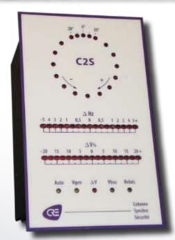
This second generation of microprocessor module combines all the visualization and control functions needed to couple a generator to a bus bar manually: display of the phase, frequency and voltage differences, a safety relay which monitors these three parameters and indicates the status of the installation.
