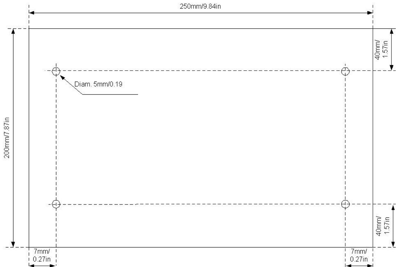
FIGURE 2 · GENSYS 2.0 CORE MOUNTING DIMENSIONS
