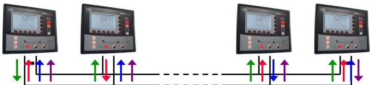
FIGURE 80 - BROADCASTING DATA BETWEEN MULTIPLE UNITS
