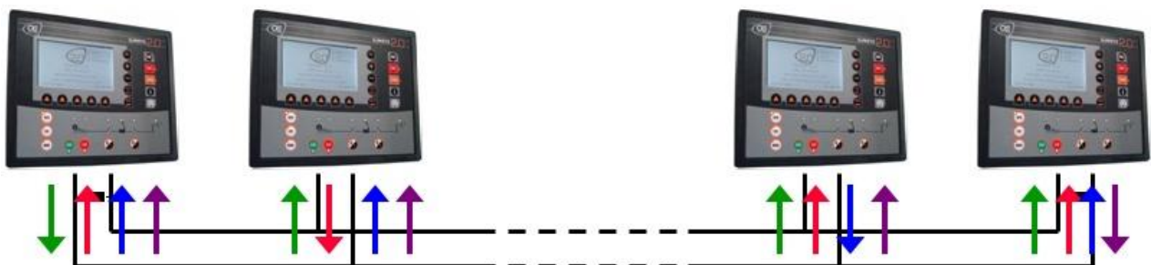
FIGURE 80 - BROADCASTING DATA BETWEEN MULTIPLE UNITS
