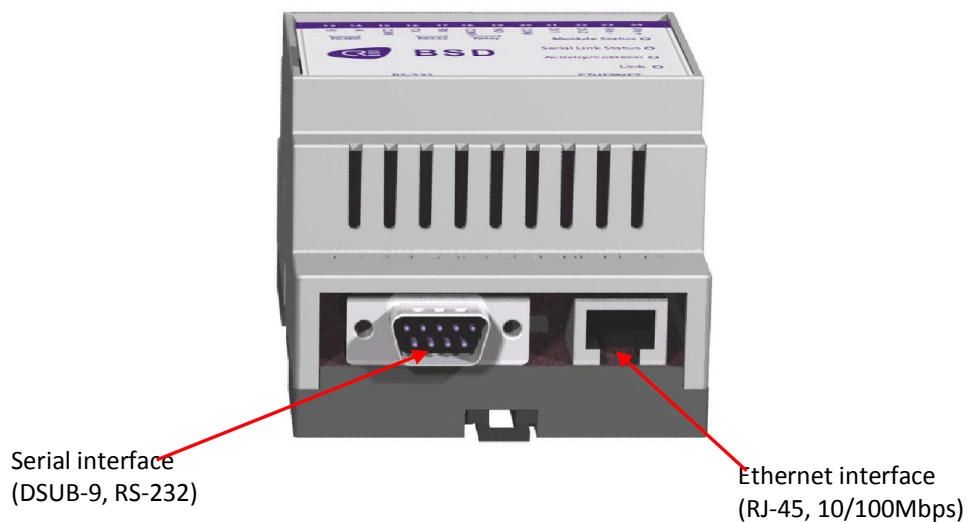
Figure 3 : DSUB-9, RS-232 and Ethernet Interfaces
