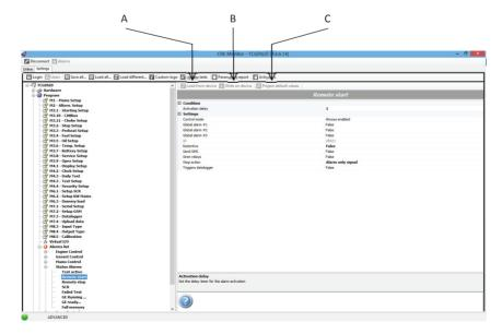
To complete the downloading of the modified parameters, press «Write on device» (A).
